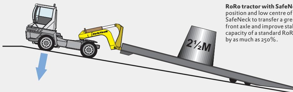
**RoRo tractor with SafeNeck:** forward mounting position and low centre of gravity. This enables the SafeNeck to transfer a greater load to the tractor front axle and improve stability. The safe working capacity of a standard RoRo tractor can be increased by as much as 250%.
