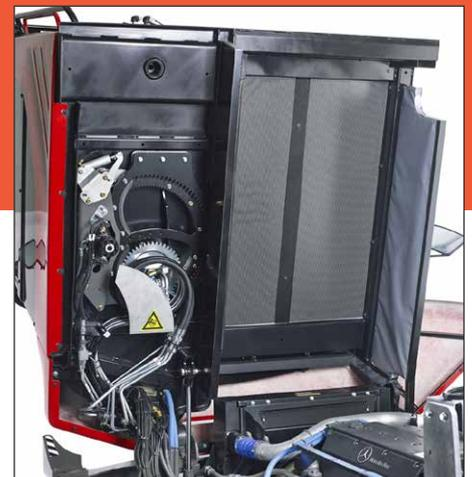
Standard feature: sound insulation material to ensure low noise level
