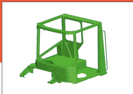
All-steel cab structure (FOPS and ROPS tested)
