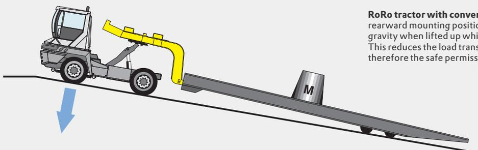
**RoRo tractor with conventional gooseneck:** rearward mounting position and high centre of gravity. This reduces the load transfer to the front axle and therefore the safe permissible payload.
